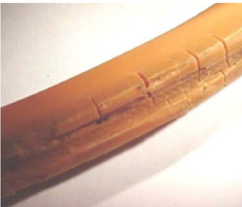
Above: Thermoplastic elastomer seal in the late stages of hydrolysis.
