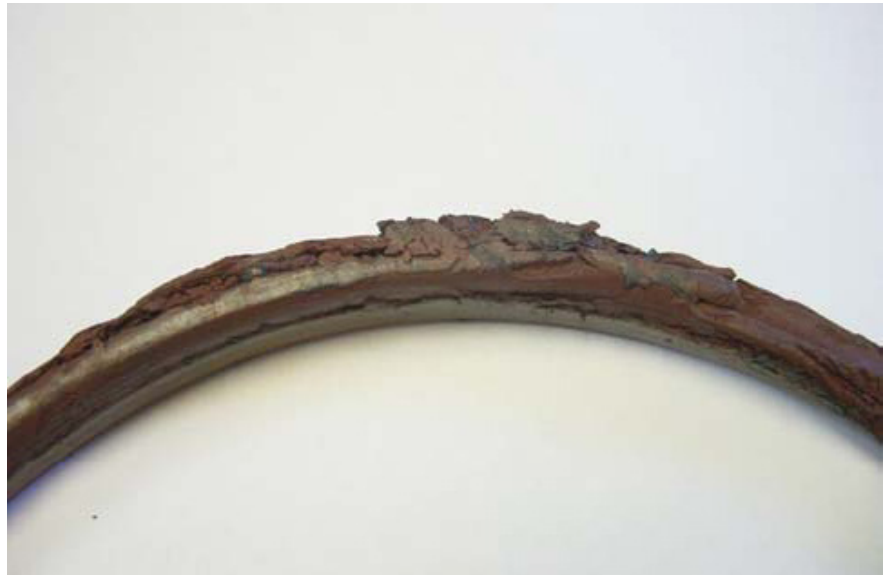
Above: Fluorocarbon (FPM) seal showing late stages of hydrolysis.
