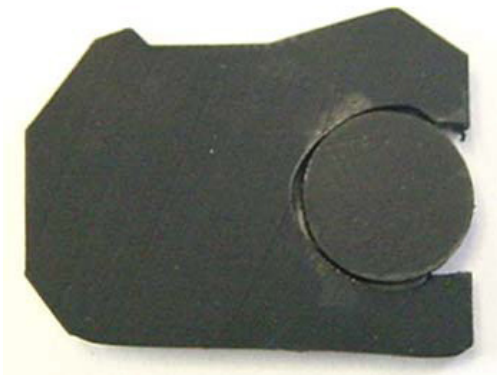
Above: Section profile of the above seal showing wear and loss of pre-load. Note both dynamic lips (bottom lips) have lost their sharp edges and have flattened compared to the top lips.
