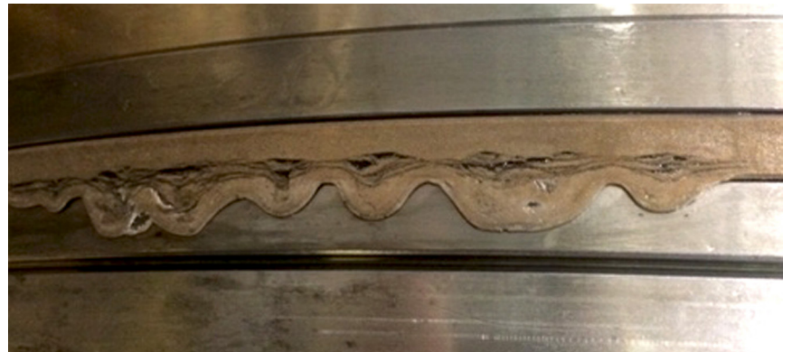
Above: PTFE piston seal showing signs of severe extrusion.
