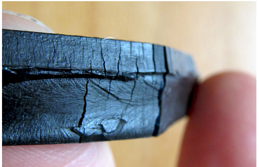
Above: Polyurethane u-cup seal with severe heat damage/cracking.
