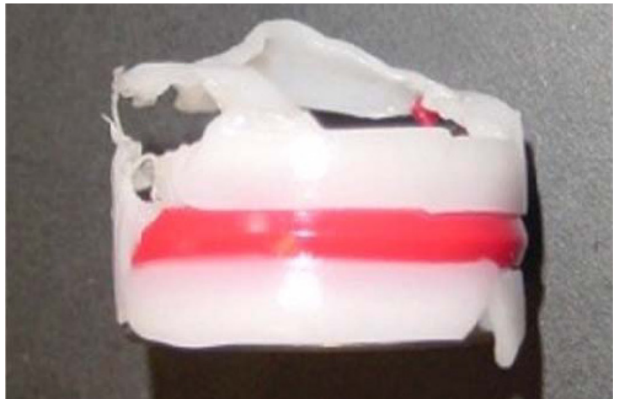
Above: Multi-component piston seal exposed to temperatures that caused the components to melt.
