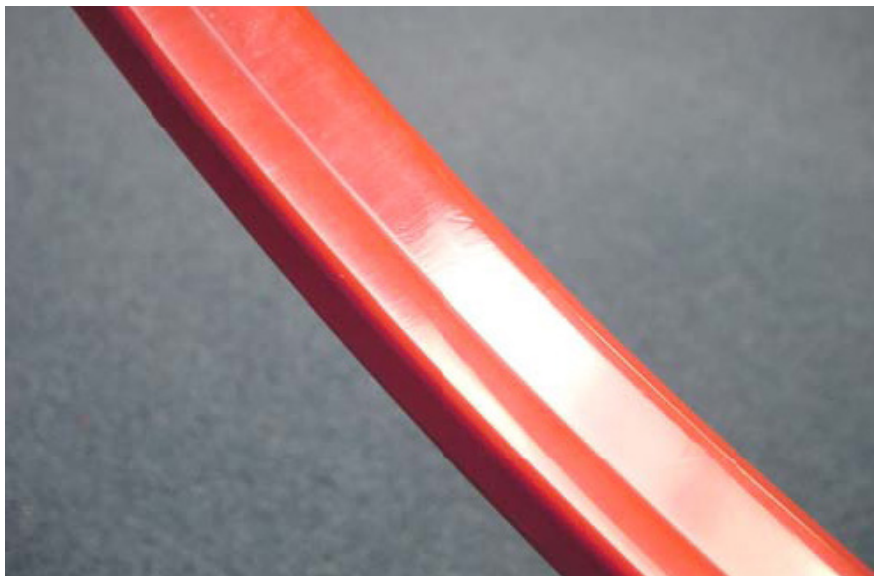
Above: Polyurethane rod seal with shiny and smooth surface from a dry running condition.
