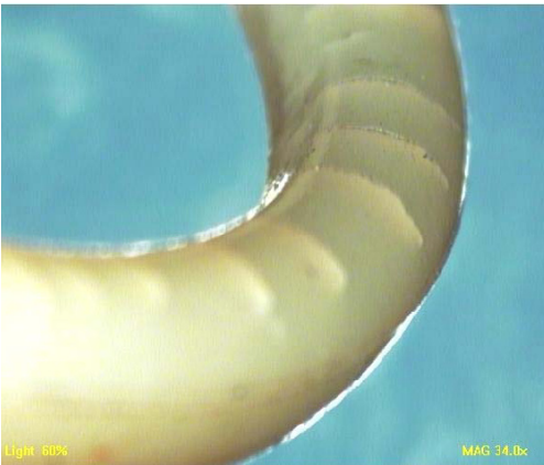
Above: Polyurethane o-ring showing early signs of hydrolysis.
