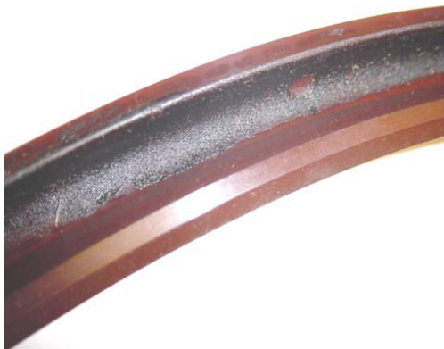
Above: Polyurethane u-cup with dieseling damage.
