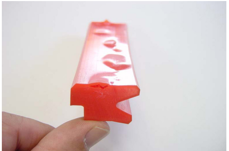
Above: Polyurethane u-cup seal damaged by explosive decompression.
