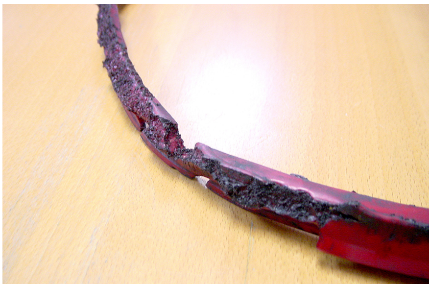
Above: Polyurethane u-cup showing severe dieseling damage.
