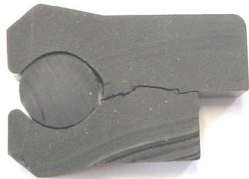
Above: Profile section of an o-ring loaded u-cup with flex fatigue cracking.
