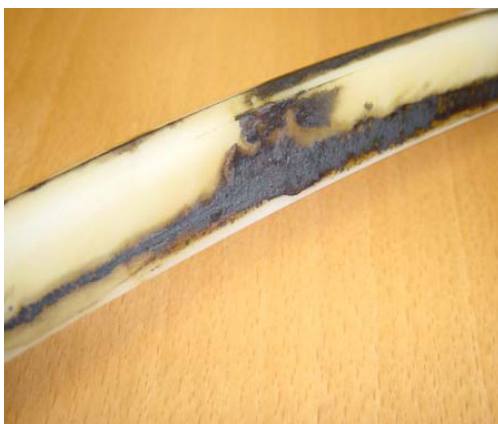
Above: Nylon back-up ring with dieseling damage.
