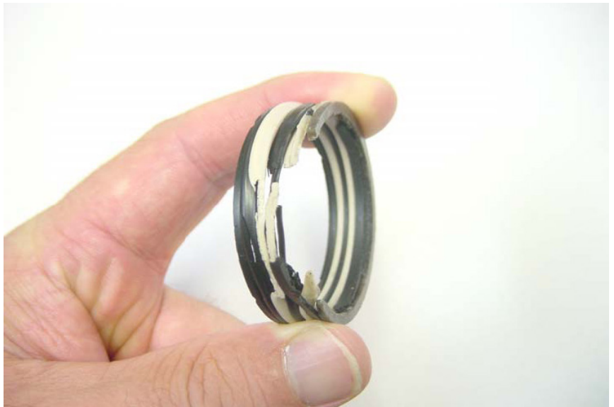
Above: V-packing set that structurally failed at 115,000psi.
