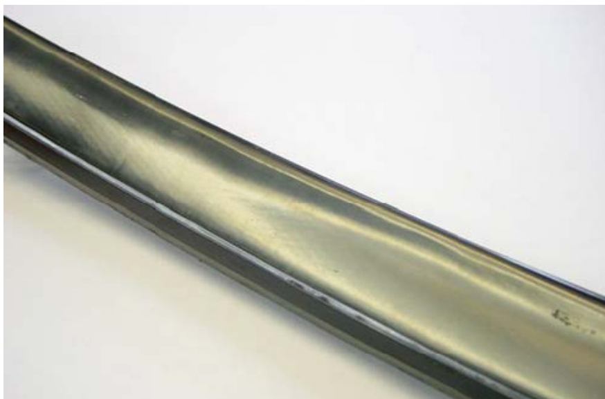
Above: NBR rod seal with shiny and smooth surface from low lubrication (water-based fluid).
