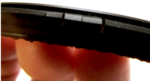
Above: Inner lip of a nitrile rotary shaft seal that has cracked from high running temperatures.
