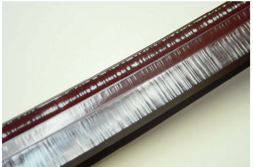
Above: Severe flow erosion of a polyurethane rod seal. Note the erosion starts at the seal lip (bottom) and migrates all the way across the seal.
