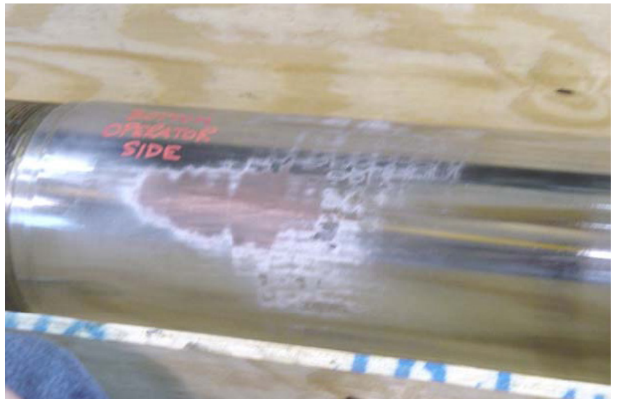
Above: Side loading that wore the chrome off the rod.
