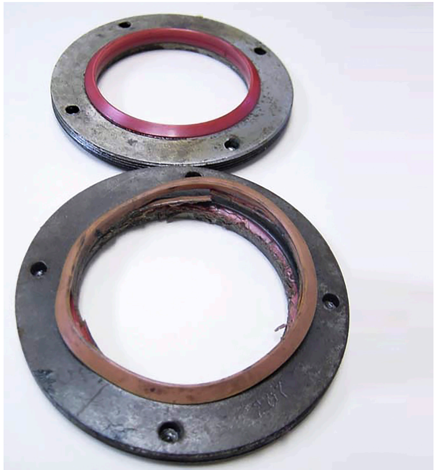
Above: Swelling failure of a dirt wiper. Wiper at top is new for comparison.
