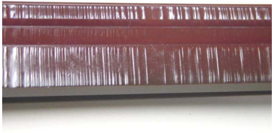
Above: Another view of the above polyurethane rod seal. Main seal lip is at the bottom.
