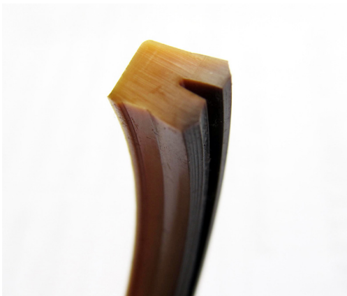
Above: Polyurethane u-cup seal with severe heat damage/cracking.
