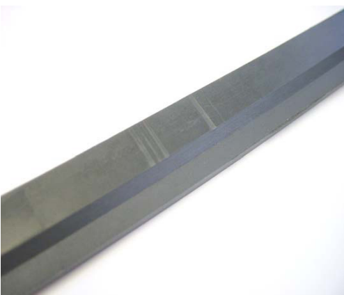
Above: PTFE seal with abrasion marks at the seal lip and migrating across the dynamic surface.
