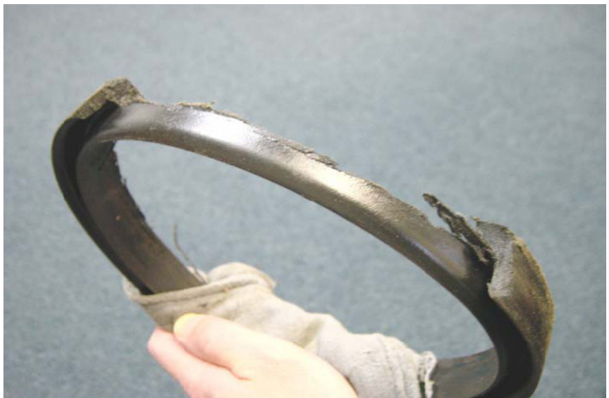
Above: Rubber and fabric piston seal that failed from over-pressurization
