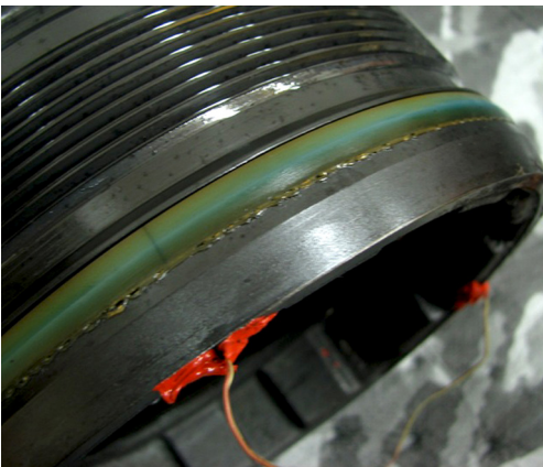
Above: Polyurethane static seal showing signs of extrusion.
