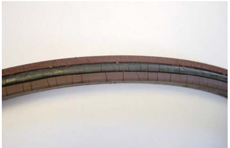
Above: Fluorocarbon (FPM) seal showing early signs of hydrolysis.
