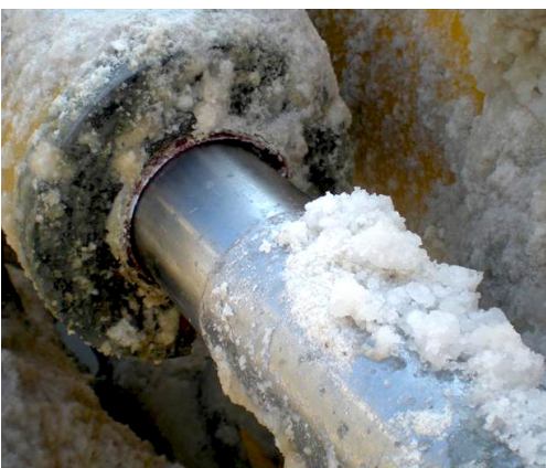
Above: Hydraulic cylinder operating in a severe salt contaminated environment.
