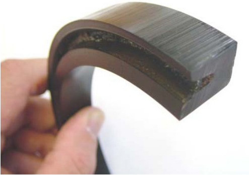
Above: NBR piston u-cup with abrasion marks at the seal lip and migrating across the dynamic surface.
